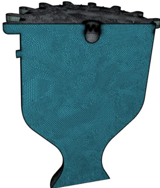
**Figure 2: Engine Model with Fine Polyhedral Mesh**
