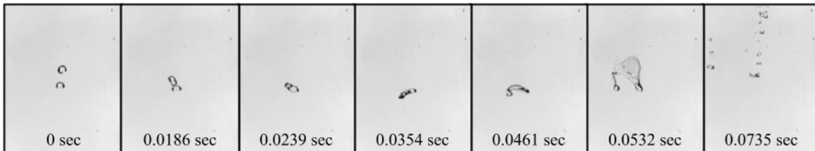
**Fig. 7 N0 drop on N0 drop collision and break-up.**
