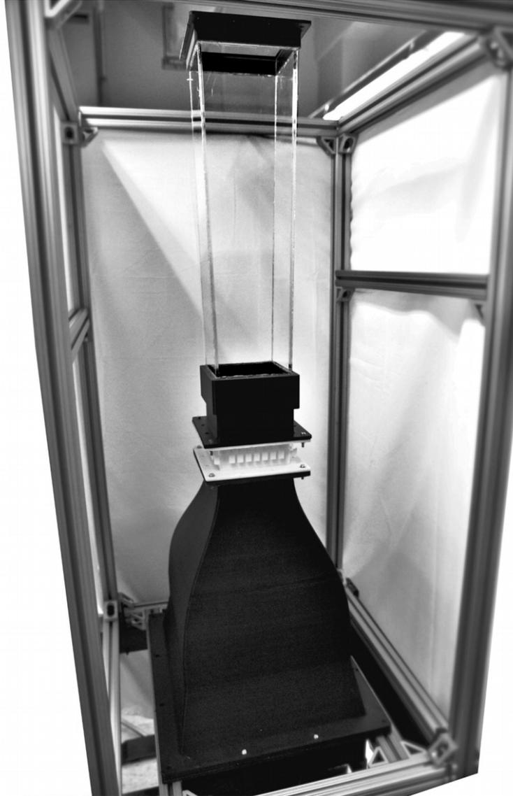
**Fig. 1 Vertical wind tunnel used for initial experiments.**
