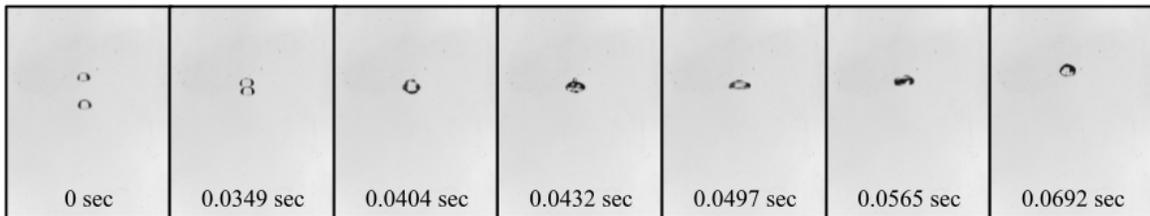
**Fig. 6 N0 drop on N0 drop collision and coalescence.**
