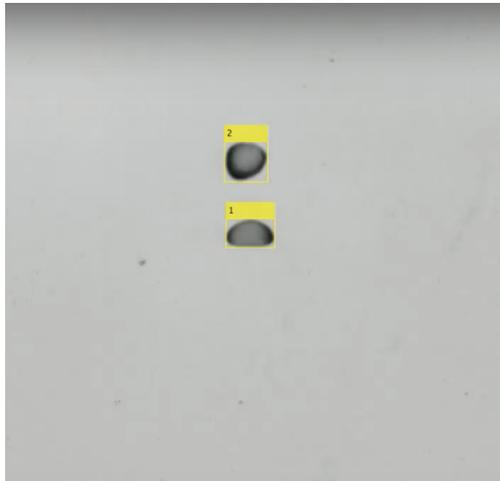
**Fig. 4 Drop collision tracking system monitoring drops within a video.**
