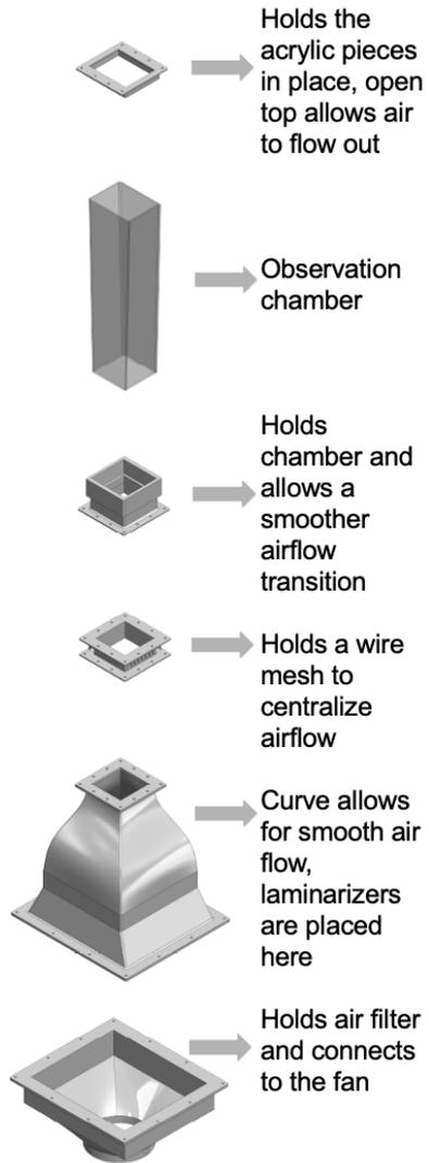
**Fig. 2 Vertical wind tunnel disassembled with part descriptions from Sebek et al. [15].**
