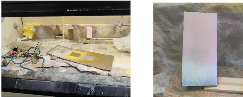
Fig. 3 Fume Hood for PSP Airbrush Painting and Wedge Model for PSP Applications
