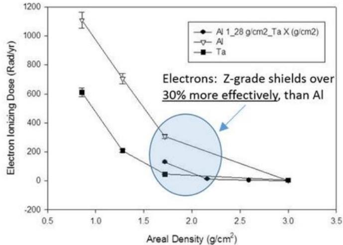
Fig. 1 Modeled ionizing dose for Al, Ta, and Al/Ta (Z-grade) samples as a function of their areal densities [7].
