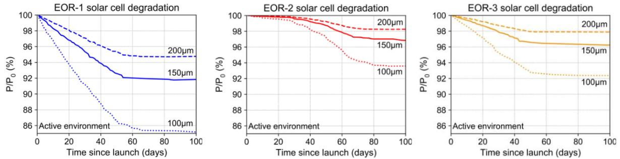
**Fig. 2 Remaining power output for a solar cell depending on its orbital path (depicted by EOR-1, EOR-2, or EOR-3) and thickness of coverglass used after exposure to a nonionizing dose for 100 days. EOR = electric orbit raising [8].**
