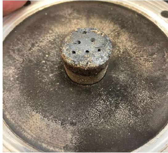
**Fig. 11 Inspection of Injector Post Launch.**
