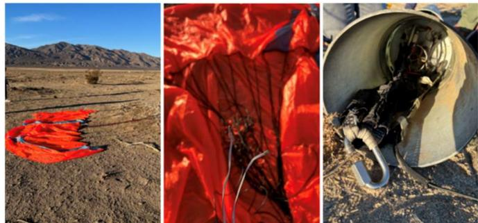
When the vehicle was recovered after launch, a large tear in the parachute along one of the seams
