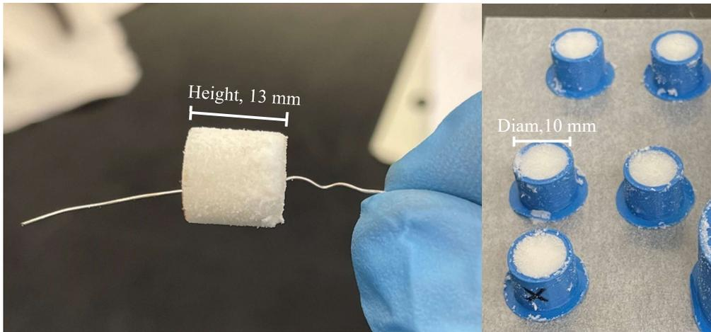
**Figure 5: Propellant General Shape and Dimensions**
