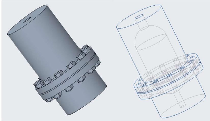
**Figure 6: Combustion Chamber Solid Model (Left) and Wireframe (Right)**
