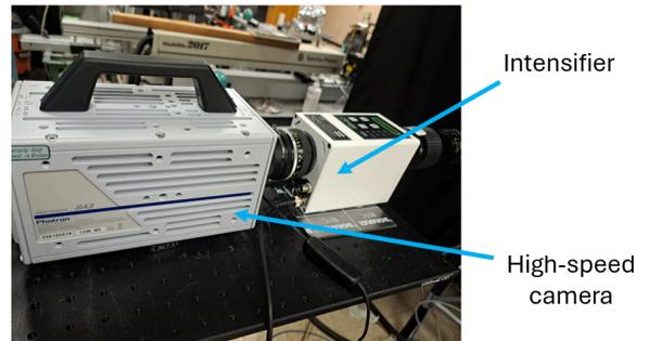
**Fig. 5: CI setup consisting of a high-speed camera and intensifier**
