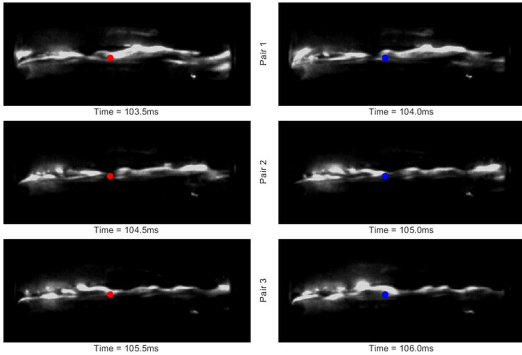
**Fig. 6: Chemiluminescence Imaging of paraffin wax boundary layer combustion [4]**
