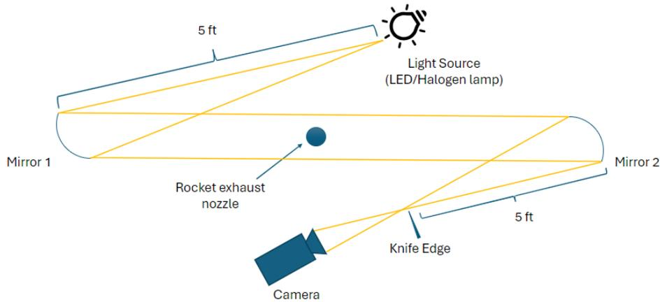
**Fig. 4: Traditional Schlieren Imaging setup**
