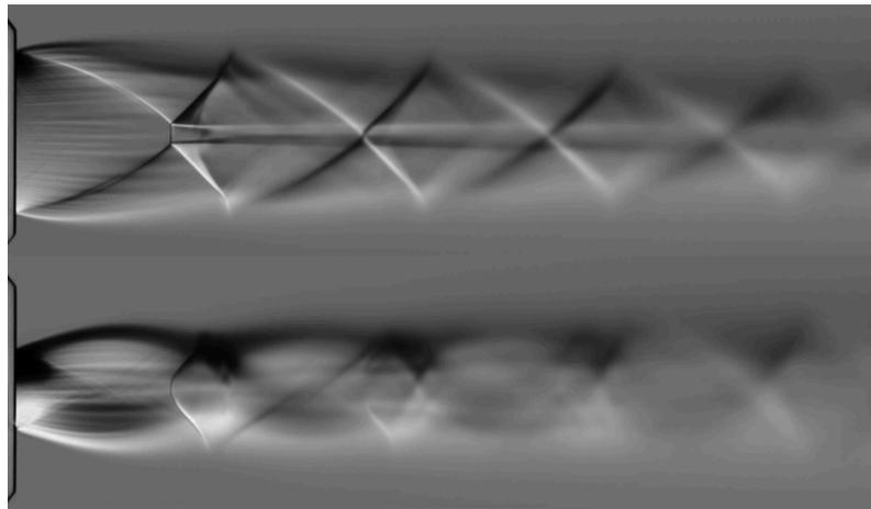
**Fig. 3: Traditional Schlieren image of underexpanded elliptical jet [6]**
