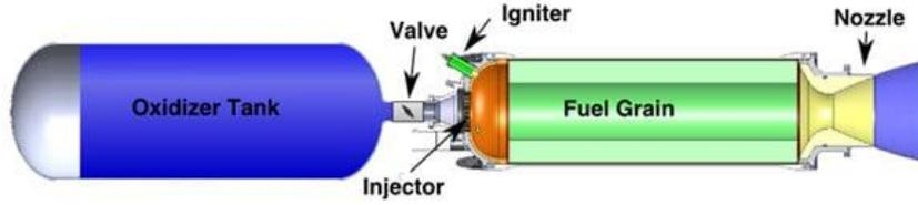
**Fig. 1: Schematic of hybrid rocket engine [6]**
