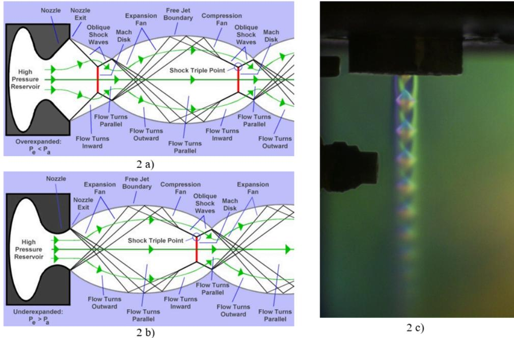
**Fig. 2: a) Overexpanded exhaust plume, b) Underexpanded exhaust plume structure [7], c) FCS Imaging of mach diamonds [8]**
