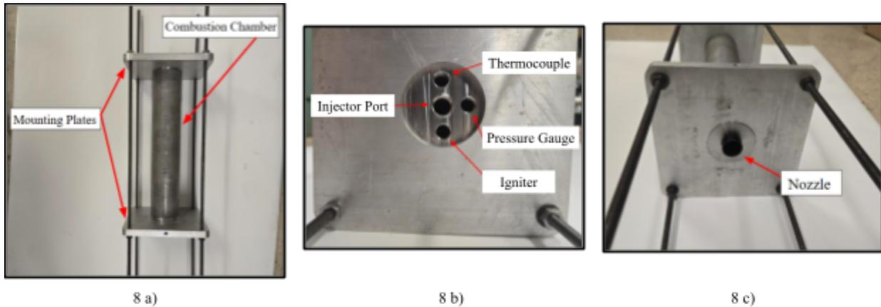
Fig. 8: a) Hybrid Rocket Combustion Chamber, b) Combustion Chamber Upstream End, c) Combustion Chamber Downstream End
