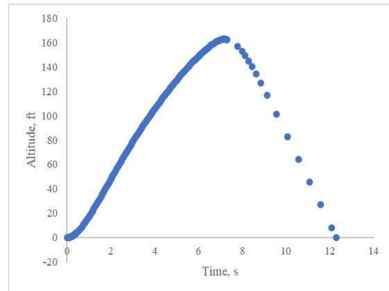
**Figure 8. Altitude of Vector as a function of time.**
