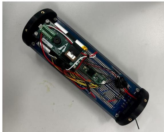
**Figure 4: Fully Integrated Avionics Bay**
