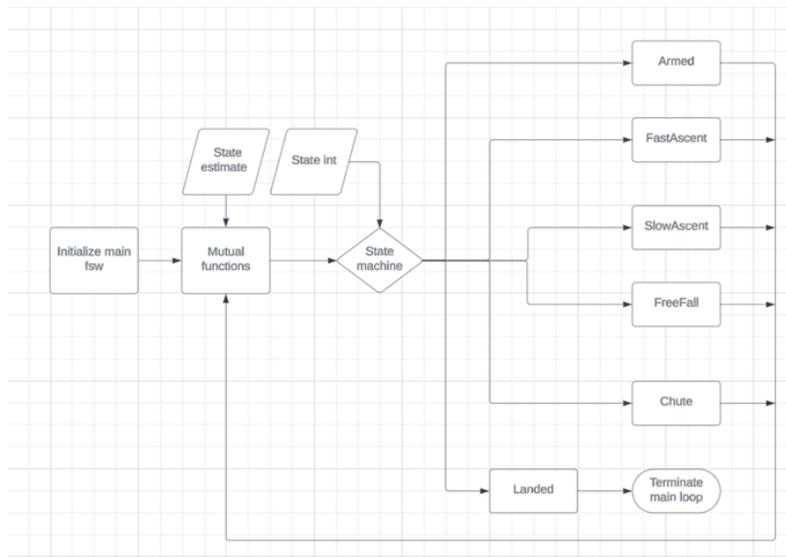
**Figure 2: Flight Software Architecture**
