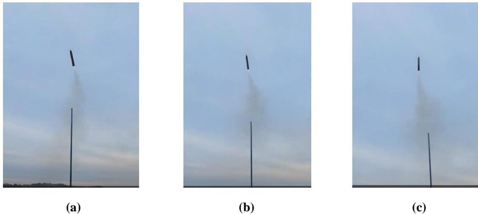
**Figure 12. Rocket Flight Over 0.5 Second Window Showing Correction in Vertical Orientation**
