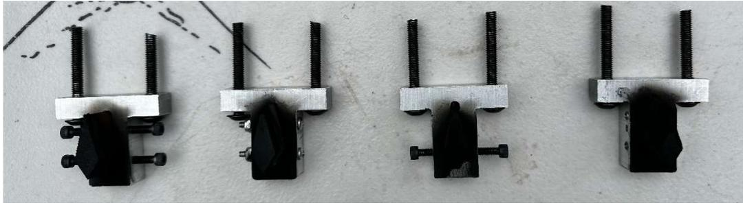
Fig. 5: Vanes after first static fire. Tungsten Carbide, Tungsten Copper, Steel, Graphite
