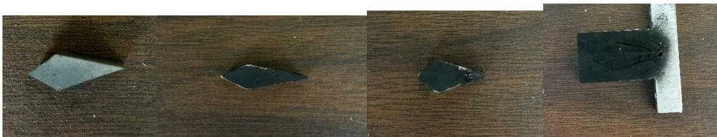
Fig .6: Vanes after second static fire. Tungsten Carbide, Tungsten Copper, Steel, Graphite
