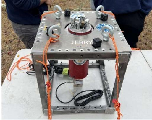
**Fig. 1: Assembled 54mm Test Stand**
