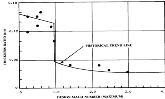
Fig. 3 Design Mach number vs thickness to chord ratio [6].
