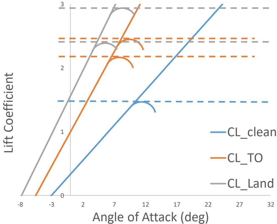
**Fig. 4 Lift coefficient vs. angle of attack.**
