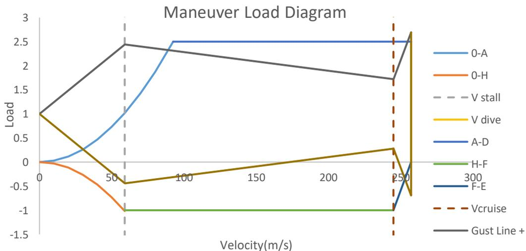
**Fig. 5 Maneuver and gust loading diagram.**
