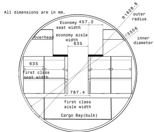
**Fig. 2 Fuselage cross-section.**
