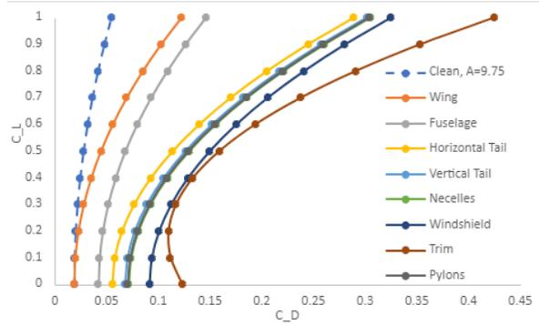
**Fig. 8 Component-wise drag polar.**
