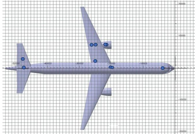
**Fig. 6 Component wise CG breakdown.**
