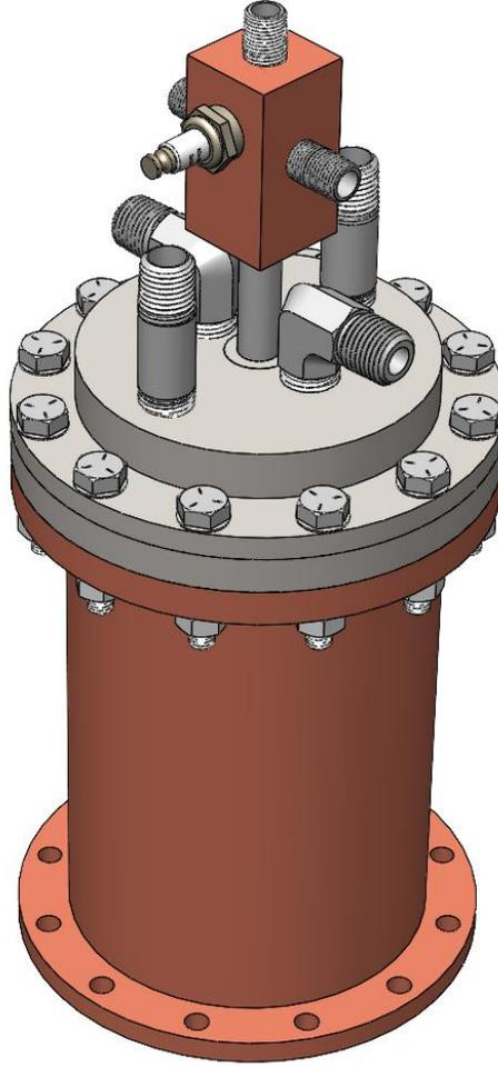
Fig 3. Igniter Integrated with the “Prometheus” Engine
