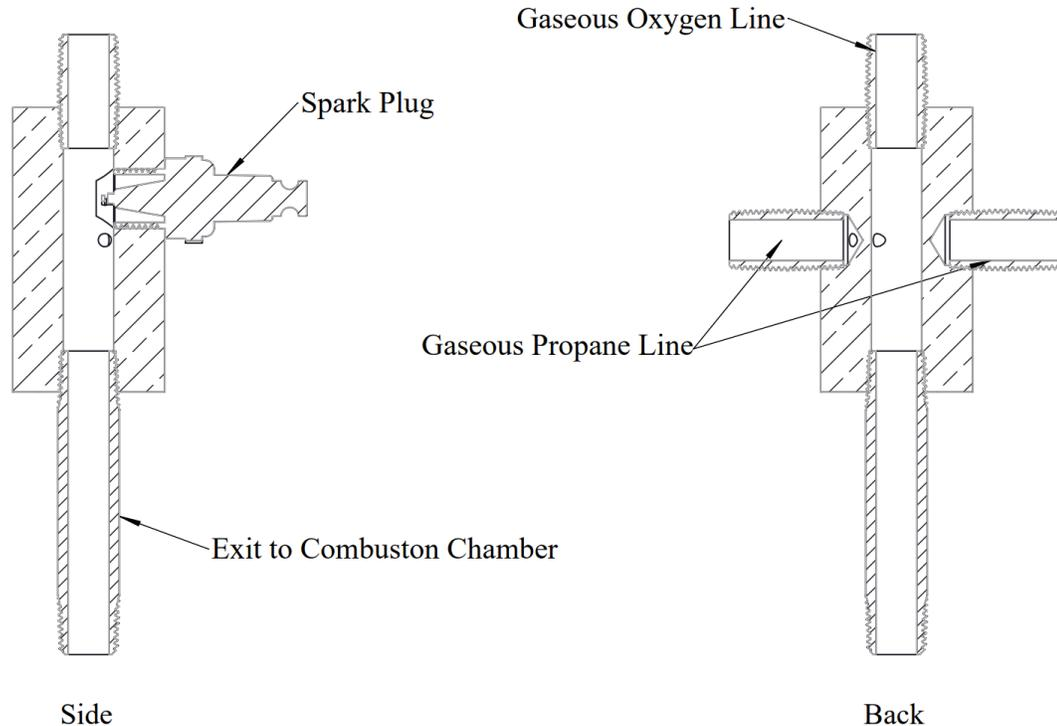
**Fig. 2 Current Torch Igniter Design Sectional View**
