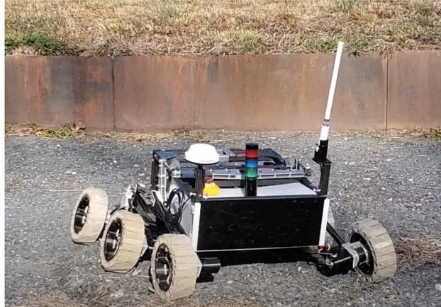
**Fig. 2 Demonstration of legs bowing in Wall-I.**
