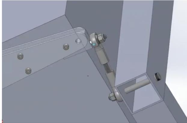
**Fig. 5 Alternate design of linkage-leg connection.**
