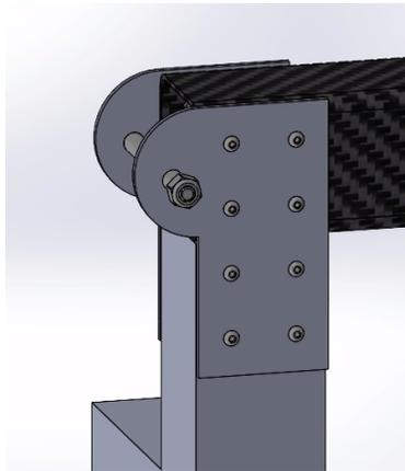
**Fig. 8 P-shaped gussets for linkage-leg connection.**
