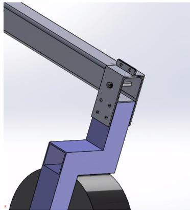
**Fig. 6 Clamp design of linkage-leg connection.**
