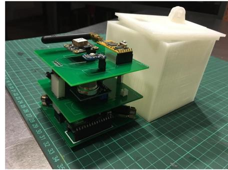
**Fig. 11** Photograph of the real CAPO prototype. The 3D-printed Cube includes a piece to attach the prototype to a drone.
