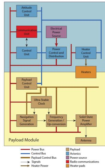
Fig. 6 NAVSAT block diagram.
