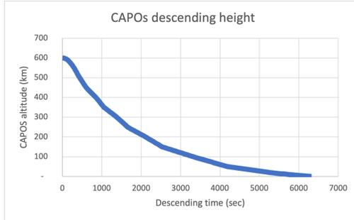
**Fig. 9** Graph of the calculated altitude vs time.
