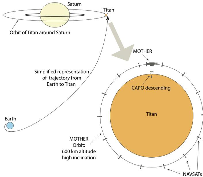
**Fig. 2 System diagram. Shows the Mission concept and its main components.**
