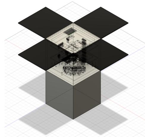
**Fig. 8** Representation of the CAPO while descending. The white cube is the payload (what we have prototyped), the grey cube is the propulsion unit and the black plates are the deployable flaps.
