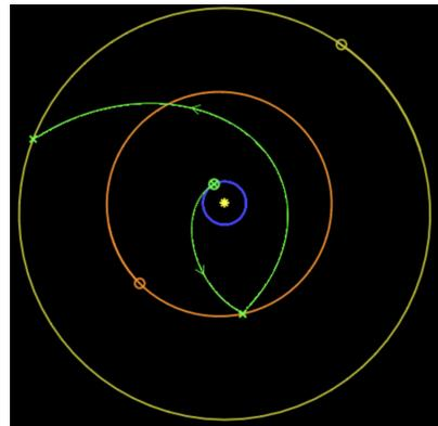
Fig. 4 Proposed trajectory, from Earth to Saturn. The blue circle (actually an ellipse but almost circular) is the Earth's orbit. The next "circle", in orange, is Jupiter's orbit. The outer yellow "circle" shows the orbit of Saturn. All showing the position of launch. The green line shows the trajectory to Saturn, including a close flyby of Jupiter.
