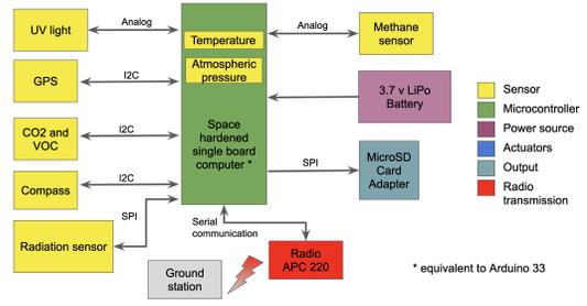
Fig. 7 CubeSat block and connexions diagram.
