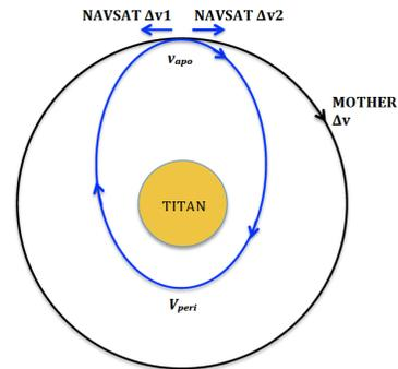
**Fig. 5 NAVSATs Hohmann transfer orbit diagram**
